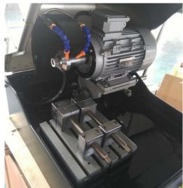
SQ-60 is suitable for cutting all kinds of specimens including metallic materials and nonmetallic materials so as to observe metallographic structure and lithofacies structure.
